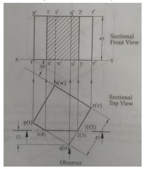
2. A cube of side 30 mm rest on the HP on one of its faces with a vertical face is inclined at 35° to the VP. It is cut by a section plane perpendicular to the VP and inclined at 35° to the HP and meeting the axis at 25 mm above the HP. Draw the front view, sectional top view and the true shape of the sections.
