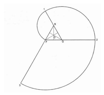
5. Draw an involute of a circle of diameter 40 mm, also draw a tangent and normal to the curve at a point 100 mm from the center of the circle.
