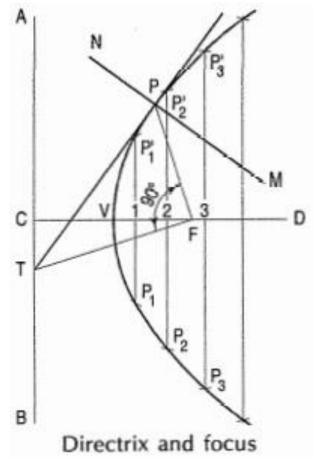
3. Infer the construction of a curve, when the distance between the focus and directrix is 50 mm and eccentricity is 3/2. Also draw the tangent and normal to any point on the curve.
