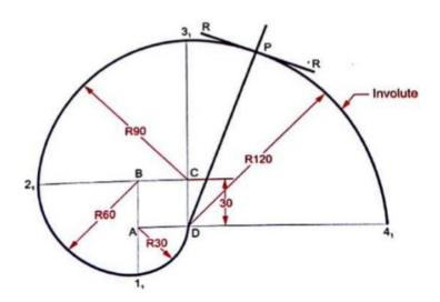
b) Draw an involute of a triangle of base side 30 mm. Also draw the tangent and normal to any point on the curve.
