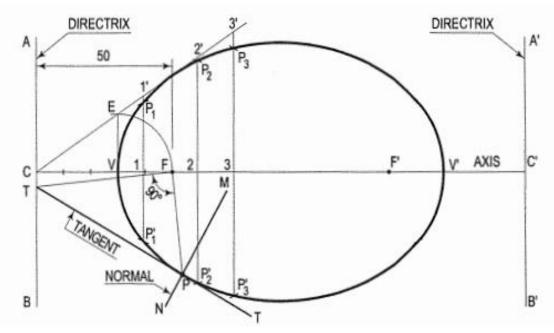
2. Infer the construction of a curve when the distance between the focus and directrix is 40 mm. The curve intersecting on axis is equidistance from fixed line and fixed point. Name the curve and draw the tangent and normal to any point on the curve.
