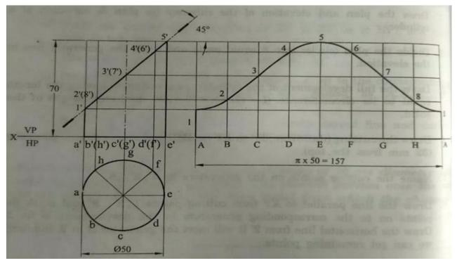
14. A cylinder of diameter 40 mm and height 70 mm is cut by a section plane perpendicular to VP and inclined at 55° to the HP meeting the axis at top face draw the lateral development of cylinder.
