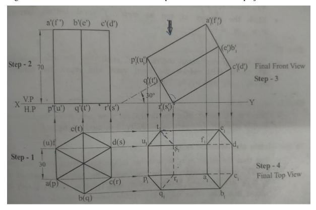
4. A hexagonal prism of base side 25 mm and axis length 50 mm rest with one of its base corners on HP. Such that the base makes an angle of 60° to HP and its axis parallel to VP. Draw its projections.
