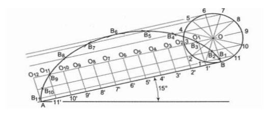
10. A ball of diameter 50 mm rolls on the outside of another ball of diameter 180 mm for one revolution. Draw the path traced by a point on the smaller ball.
