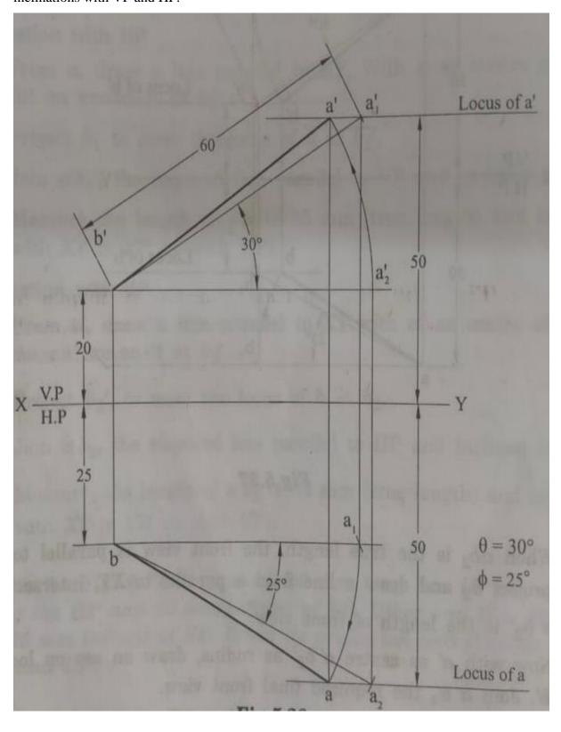
6. A line AB 65 mm long has its end A 20 mm above HP and 25 mm infront of VP. The end B is 40 mm above HP and 65 mm infront of VP. Draw its projections and find its inclinations with VP and HP.
