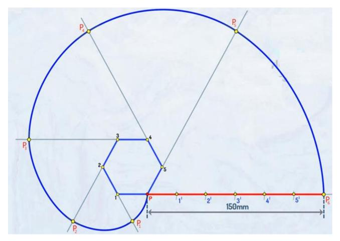
8. A coin of 40 mm diameter rolls over a horizontal table without slipping. A point on the circumference of the coin is in contact with the table surface in the beginning and after one complete revolution. Draw the path traced by the point. Also draw the tangent and normal to any point on the curve.
