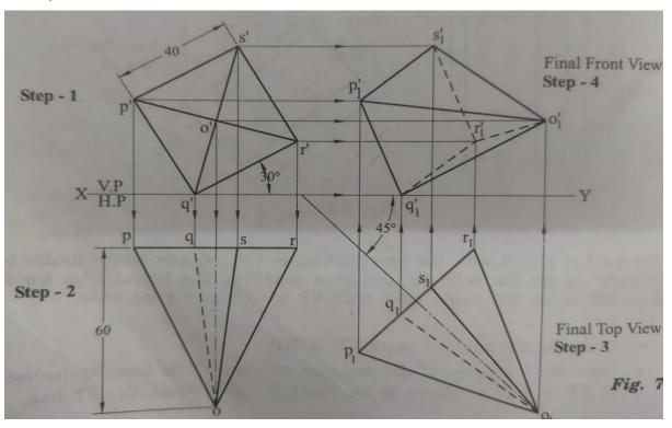
12. A square pyramid of base side 40 mm and axis 60 mm rests on the HP on one of its base edges perpendicular to VP and the triangular faces containing the resting edge is perpendicular to both VP and HP. Draw its projections.
