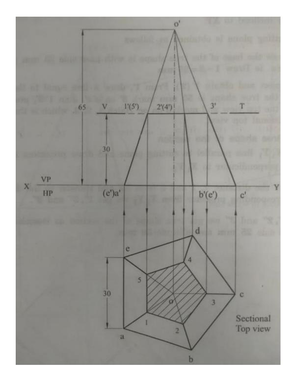
6. A hexagonal pyramid of side of base is 30 mm and altitude 65 mm long rests with its base on HP with two of its base sides are parallel to VP. It is cut by a section plane perpendicular to VP and inclined at 45° to HP and passing through the axis at a distance of 30 mm from the apex. Draw the sectional top view and true shape of the section.
