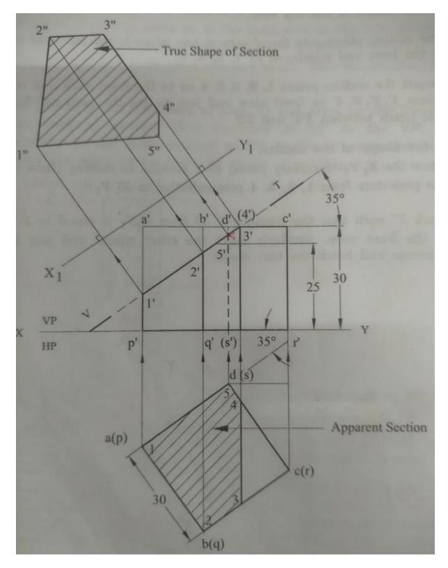
3. A hexagonal prism of side of base 30 mm and axis 75 mm long resting on its base on HP such that a rectangular face is parallel to VP. It is cut by section plane perpendicular to VP and inclined to HP. The sectional plane is passing through the top of an extreme lateral edge of the prism. Draw the sectional top view and true shape of the section.
