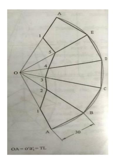
11. A hexagonal pyramid of base side 30 mm and height 60 mm resting on its base on the HP, such that two of its sides are perpendicular to VP. It is cut by section plane inclined at 40° to the HP and perpendicular to the VP. The cutting plane is bisecting the axis of the pyramid. Obtain the development of the lateral surface of the truncated pyramid.
