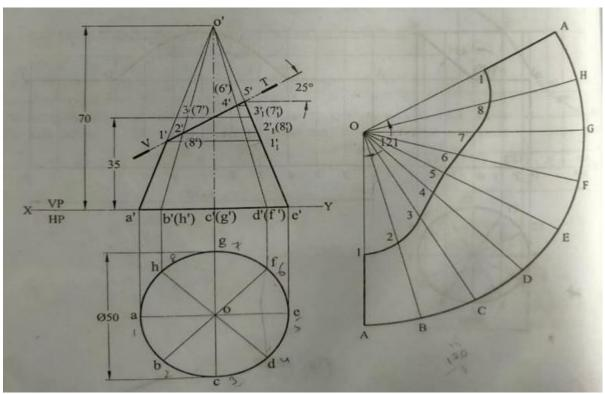
16. A right circular cone of base diameter 60 mm and height 70 mm is resting on its base on the ground. It is cut by a section plane perpendicular to VP and inclined at 30° to the HP. The cutting plane bisecting the axis of the cone. Draw the development of lateral surface of the cone.
