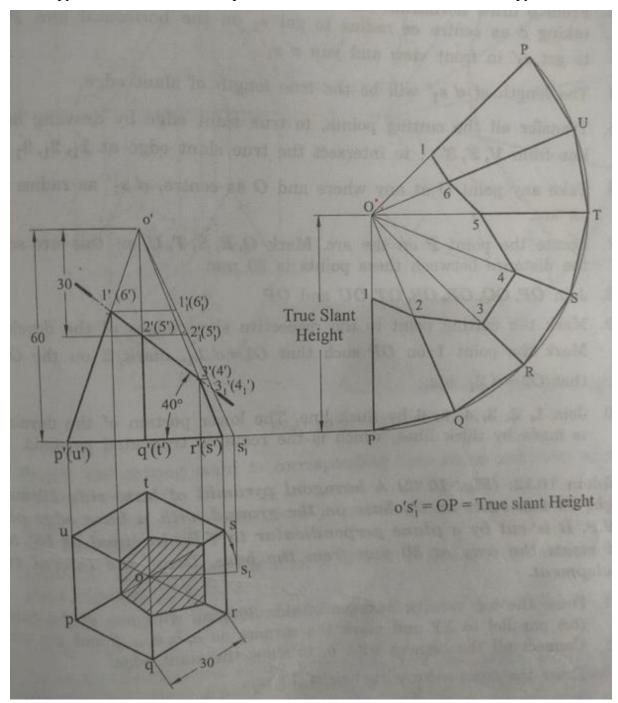
12. A hexagonal pyramid of base side 30 mm and height 70 mm rests with its base on the ground with base edge parallel to VP. It is cut by section plane perpendicular to VP and inclined at 55° to the Hpand meets the axis at 30 mm from the base. Draw the development of surfaces.
