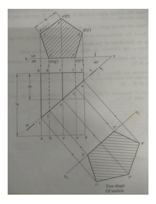
5. A pentagonal pyramid of side of base 30 mm and axis 65 mm long, rests with its base on HP and one of the edges of its base on HP and one of the edges of its base is perpendicular to VP. It is cut by a section plane perpendicular to VP. It is cut by a section plane perpendicular to VP and parallel to HP and passing through the axis at a point 30 mm above the base. Draw the front and sectional top view.
