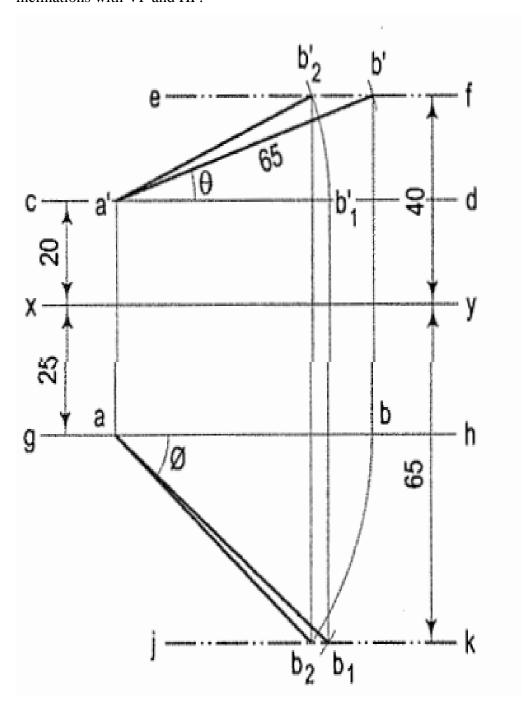
7. The distance between the projectors of two end point A and B is 70 mm. The end A is 10 mm above HP and 15 mm in front of VP. The other end B is 50 mm above HP and 40 mm in front of VP. Find the true length and true inclination using rotating line method.
