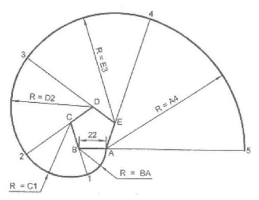
7. Draw an involute of a hexagon of base side 25 mm. Also draw the tangent and normal to any point on the curve.
