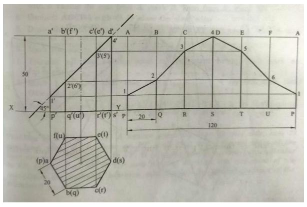
9. A hexagonal prism of base side 25 mm and height 50 mm is resting on one of its base on the HP and two of its lateral faces are parallel to VP. It is cut by a section plane perpendicular to VP and inclined at 30° to the HP. The plane meets the axis at a distance 25 mm above the base. Draw the development of lateral surface of the prism.
