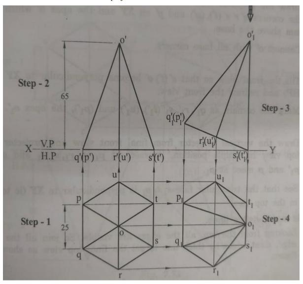
14. Draw the projection of a cone of base diameter 50 mm and axis length 60 mm, when its lies on the ground on one of its generators with the axis parallel to the VP.
