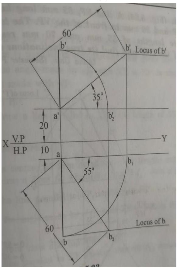
5. A line AB 60 mm long has its end B 20 mm above HP and 25 mm infront of VP. The end A is 50 mm above HP and 50 mm infront of VP. Draw its projections and find its inclinations with VP and HP.
