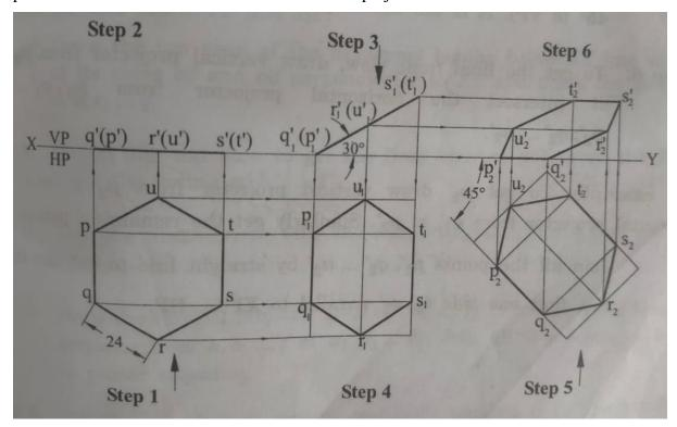
13. A regular pentagonal lamina of 30 mm sides has one edge in HP and inclined at an angle of 30° to VP. Draw its projections when its surface is inclined at 45° to HP.
